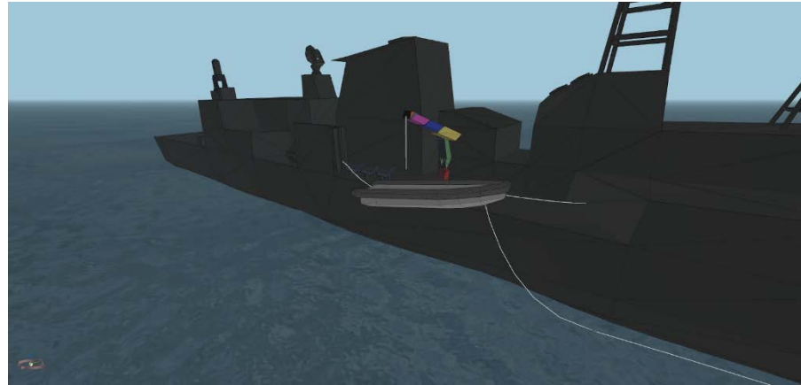
Figure 2 Simulation of the launch and recovery of a small rescue craft with a frigate. A multi-purpose boom crane is simulated. Line, crane, and pedestal loads are determined from the simulation.
